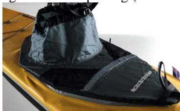
Skirt Installed over spray deck.
